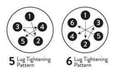
It is important to maintain proper torque specifications to provide safe and secure attachment of the wheel to the hub drum.
